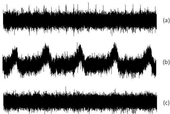
Fig. 2 Results of the removal algorithms: (a) FIR, (b) template subtraction, (c) DWT.
