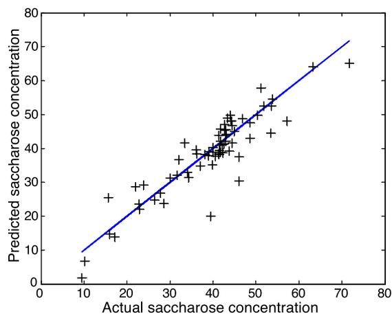
Fig. 7. Predicted saccharose concentration according to actual saccharose concentration with PLS-RBFN model for the samples of juice.
