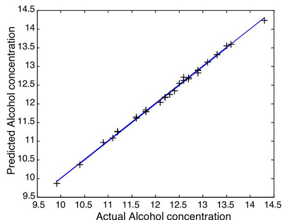
Fig. 4. Predicted alcohol concentration according to actual alcohol concentration for the wine samples with FBS-RBFN model.
