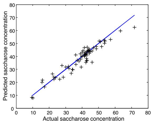
Fig. 8. Predicted saccharose concentration according to actual saccharose concentration with FBS-RBFN model for the samples of juice.
