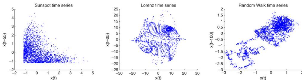
Fig. 8. Regressor distribution in a 2-dimensional space after unfolding. From left to right: Sunspot, Lorenz and random walk.
