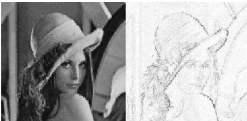
FIGURE 12 Lena image compressed without DCT, compression rate = 14.22, PSNR = 25.6 dB.
