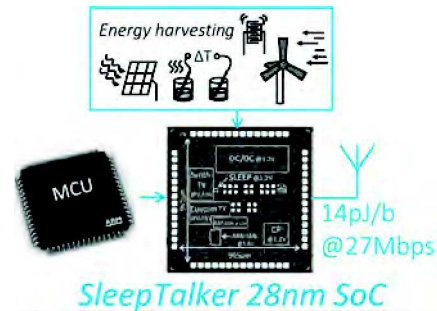
Figure 1: SleepTalker SoC microphotograph and application scenario (chip manufacturing donation from ST Microelectronics, Crolles, France).
