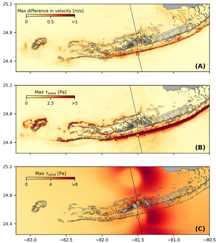
Fig. 9. (A). Maximum difference between SLIM and SLIM+SWAN currents during the passage of Irma in the Lower Florida Keys; (B) Maximum wave radiation stress gradient  $\tau_{wave}$  and (C) maximum wind stress  $\tau_{wind}$  (C) generated by the hurricane. Radiation stress gradient yields currents speed differences reaching 1 m/s, especially over offshore reefs.
