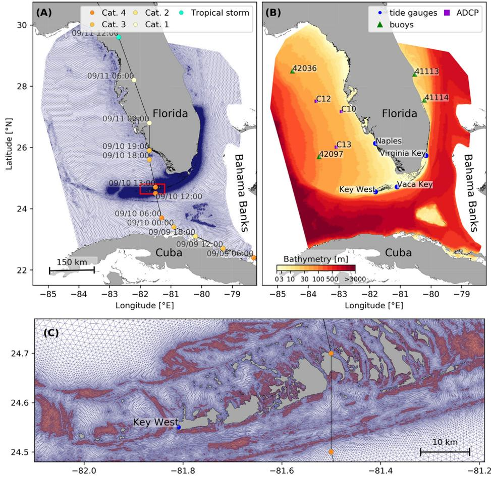
**Fig. 1.** (A) Mesh of the computational domain with the trajectory of Irma. The category of the hurricane is given by the Saffir–Simpson color scale. (B) Bathymetry of the domain with the location of stations used for the validation of the model outputs. (C) Close up view of the Lower Keys area (red box in (A)), where the mesh resolution reaches 100 m near reefs (shown in dark orange) and islands (shown in dark gray).
