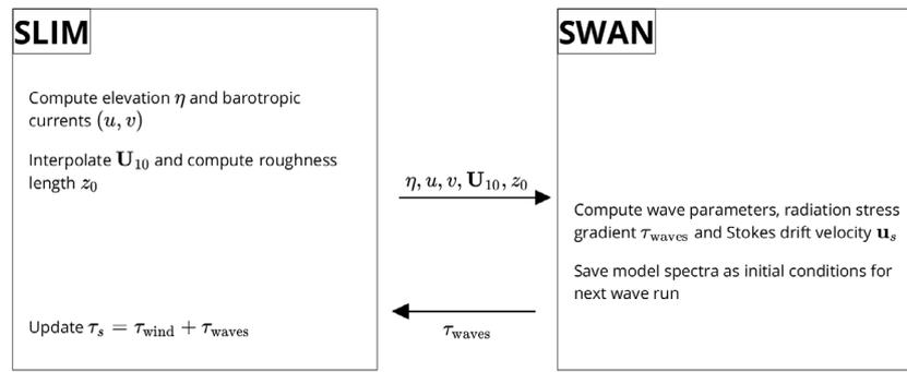
Fig. 3. Schematic illustration of the coupled SLIM+SWAN model.
