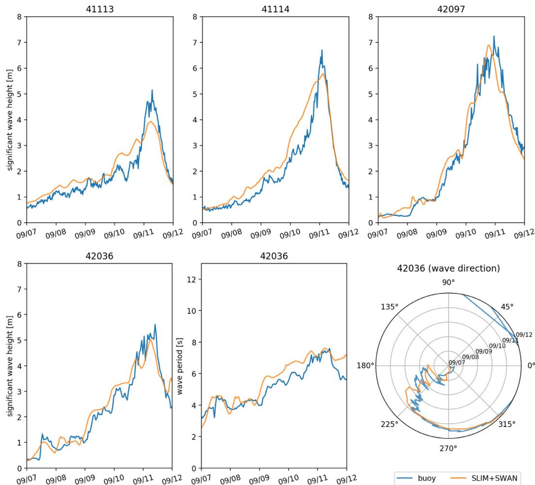
**Fig. 8.** Comparison of modeled wave parameters with observation at the 4 buoys location (locations shown in Fig. 1B). Overall, the modeled significant wave heights agree well with field measurement (mean error < 25%).
