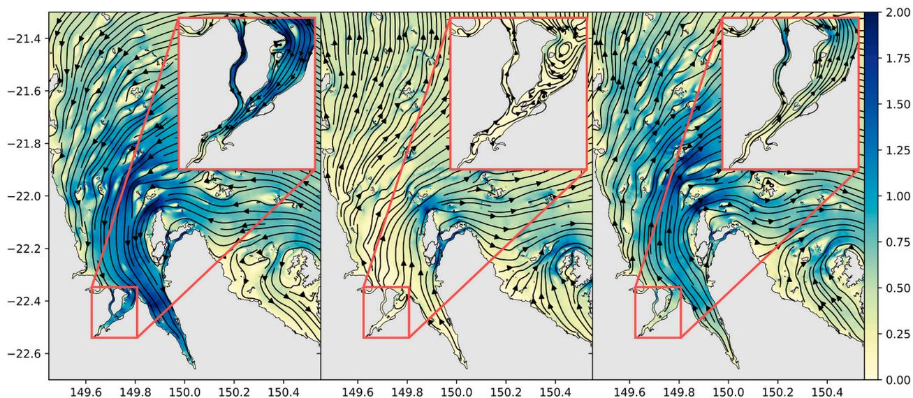
**Fig. 2.** Snapshots of SLIM outputs at three time steps, 3 h apart each (different stages of the tidal cycle). The background color represents the current magnitude in m/s and shows that currents can reach velocities up to 2 m/s at tidal peaks. Arrows represent current streamlines.
