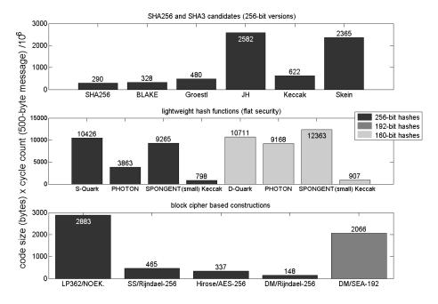
Fig. 4: Performance evaluation: code size (bytes) x cycle count (500-byte message).
