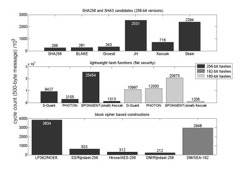
Fig. 3: Performance evaluation: cycle count (500-byte message).
