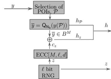
**Figure 4: The extraction process in setup mode.**
