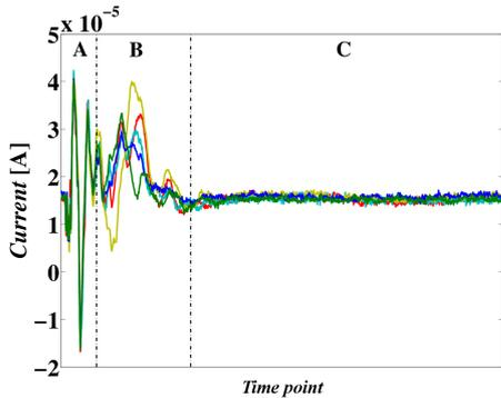
**Figure 3: Power traces of the power PUF instance showing 5 different chips using a single challenge.**
