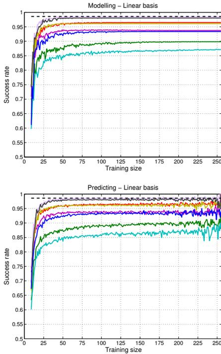
**Figure 6: Modeling and unpredictability for a single point extraction process in the PUF setup.**
