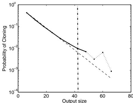
**Figure 10: Physical unclonability vs. output size after concatenating outputs of different challenges by experiments (solid) and by assuming independent outputs (dashed). The dot-dashed vertical line shows the limit posed by physical unpredictability.**
