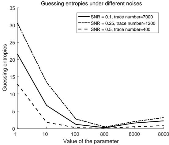
Fig. 6. The guessing entropies of non-profiled ridge-based DPA for different SNRs by varying parameter  $\lambda$ .
