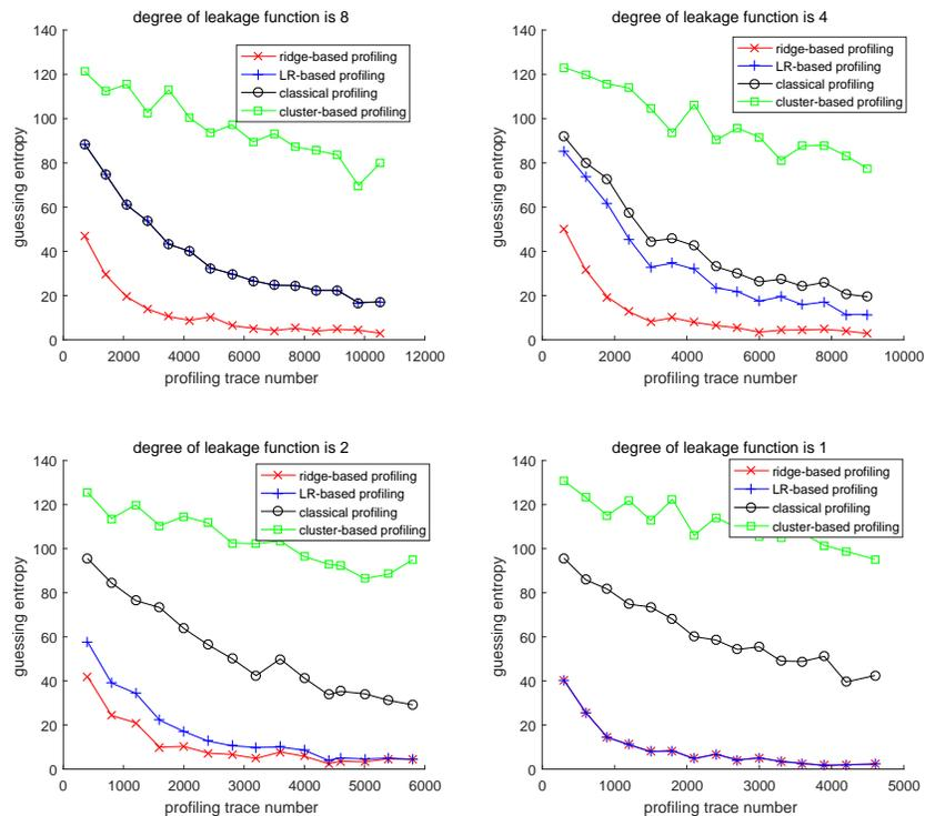
Fig. 8. The guessing entropies of profiled DPAs in a robust setting, and SNR = 0.1. We increase the number of profiling traces and fix the exploitation trace number as 2200. The upper-left, upper-right, lower-left, and lower-right figures correspond to degrees 8, 4 and 2 and 1 respectively.
