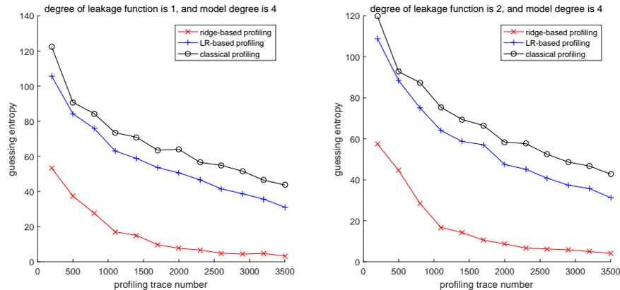
Fig. 10. The guessing entropies profiled DPAs with conservative degrees of model for different numbers of profiling traces, and the exploitation trace number is 1700, SNR = 0.1.
