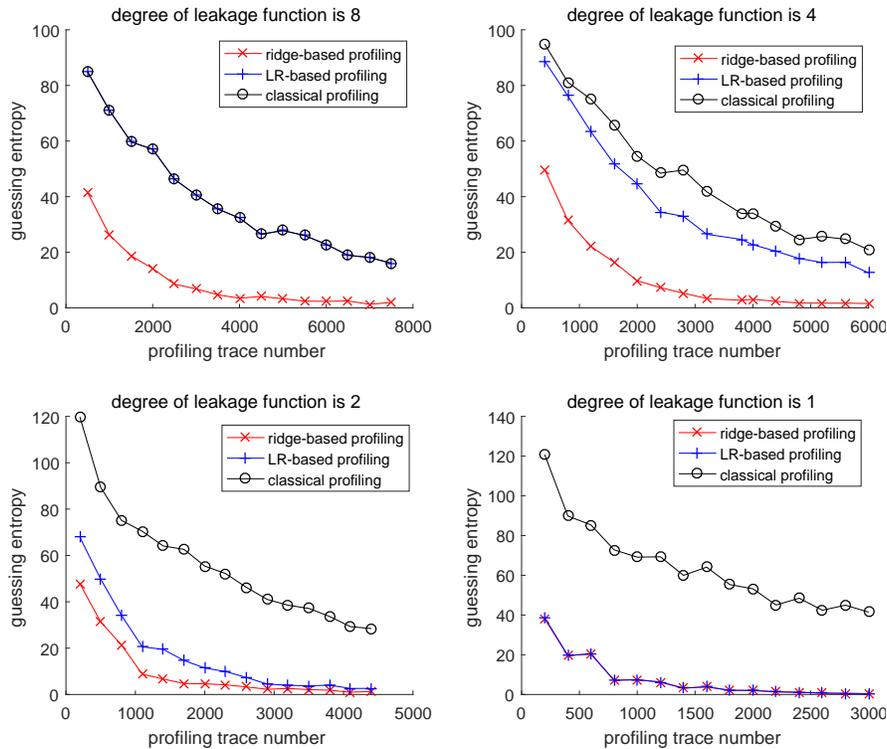
Fig. 7. The guessing entropies of profiled DPAs in the ideal setting, and SNR = 0.1. We increase the number of profiling traces and fix the exploitation trace number as 2200. The upper-left, upper-right, lower-left, and lower-right figures correspond to degrees 8, 4 and 2 and 1 respectively.
