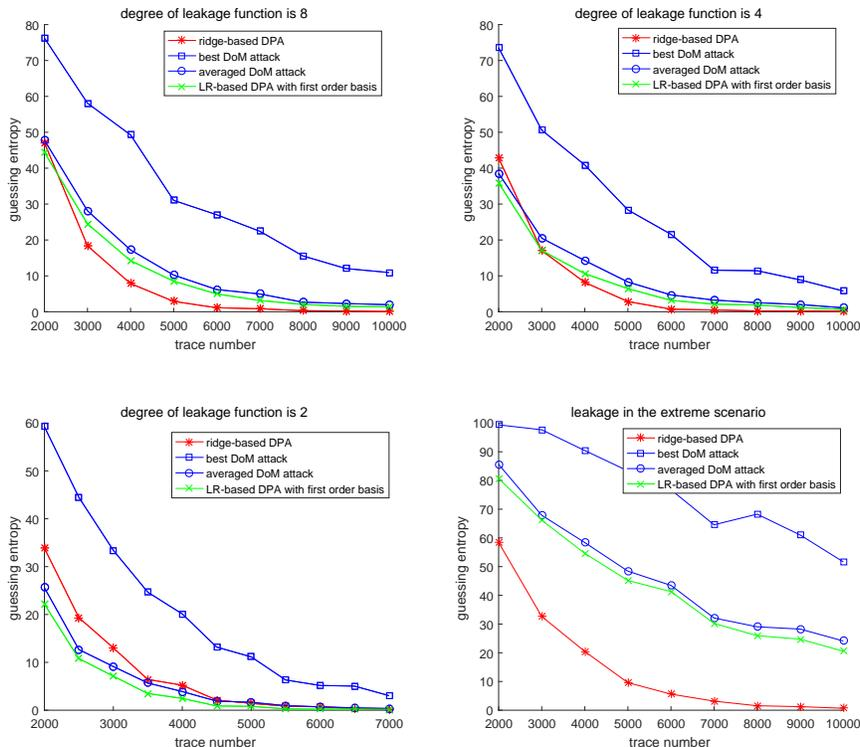
Fig. 11. The guessing entropies of non-profiled DPAs, and SNR = 0.1. The upper-left, upper-right, lower-left, and lower-right figures correspond to degrees 8, 4, 2 and the extreme case respectively.
