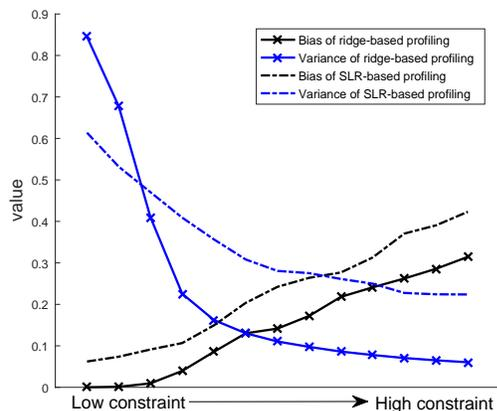
Fig. 17. The bias-variance tradeoff of SLR-based and ridge-based profilings for degree 4 in simulation-based experiments. We set SNR to 0.4, and the profiling trace number is 2000.
