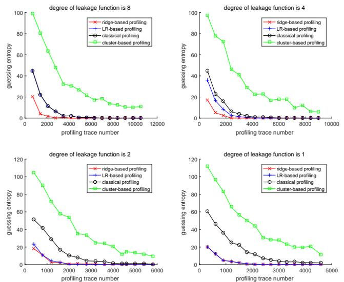
Fig. 18. The guessing entropies of the profiled DPAs of simulation-based implementation with more profiling traces, and exploitation traces number is 20000, SNR = 0.1.
