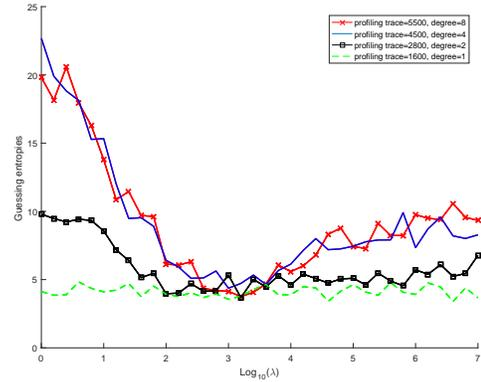
Fig. 9. The guessing entropies profiled DPAs with increasing value of  $\lambda$ , exploitation trace=1700, SNR = 0.1
