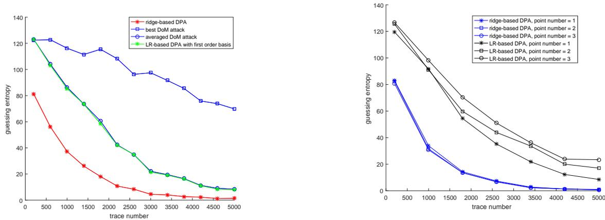
Fig. 15. The guessing entropies of the non-profiled DPAs in the FPGA-based experiments.
