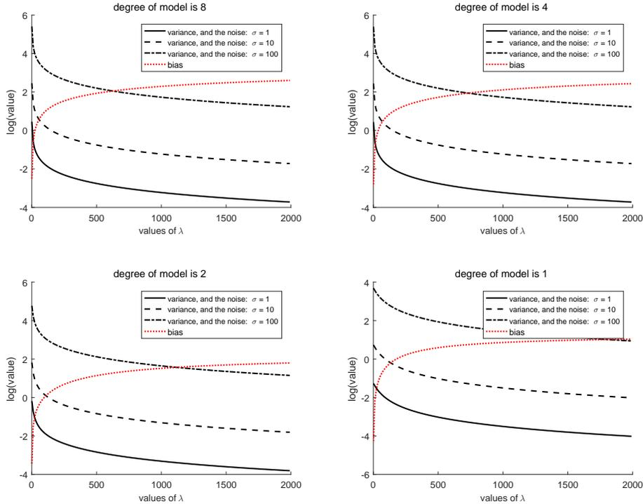
Fig. 2. The bias-variance tradeoff of ridge-based profiling for different degrees (of the model). The upper-left, upper-right, lower-left, and lower-right figures correspond to the cases for  $d = 8$ ,  $d = 4$ ,  $d = 2$ , and  $d = 1$  respectively.
