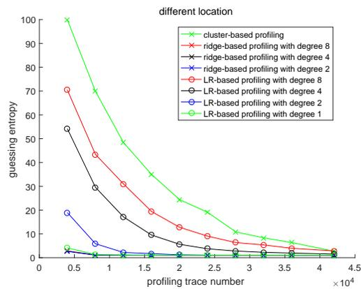
Fig. 19. The guessing entropies of the profiled DPAs in 2nd setting of FPGA implementation with more profiling traces, and exploitation traces number is 15000.
