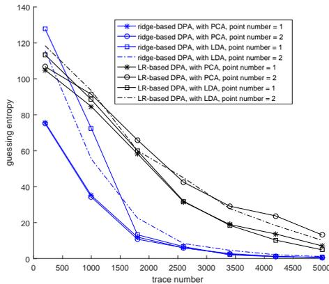
Fig. 21. The comparison of LDA and PCA in non-profiled case.
