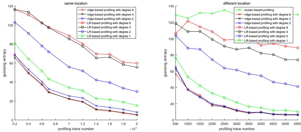
Fig. 13. The guessing entropies of the profiled DPAs in the FPGA-based experiments. Left: 1st setting. Right: 2nd setting
