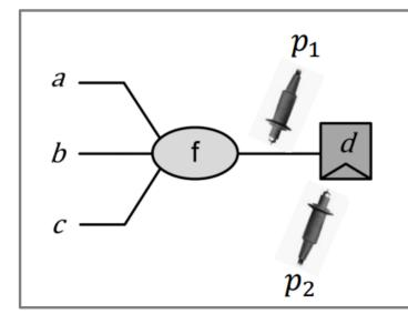
**Glitch-extended probes:** probing any output of a combinatorial subcircuit allows the adversary to observe all the sub-circuit inputs
