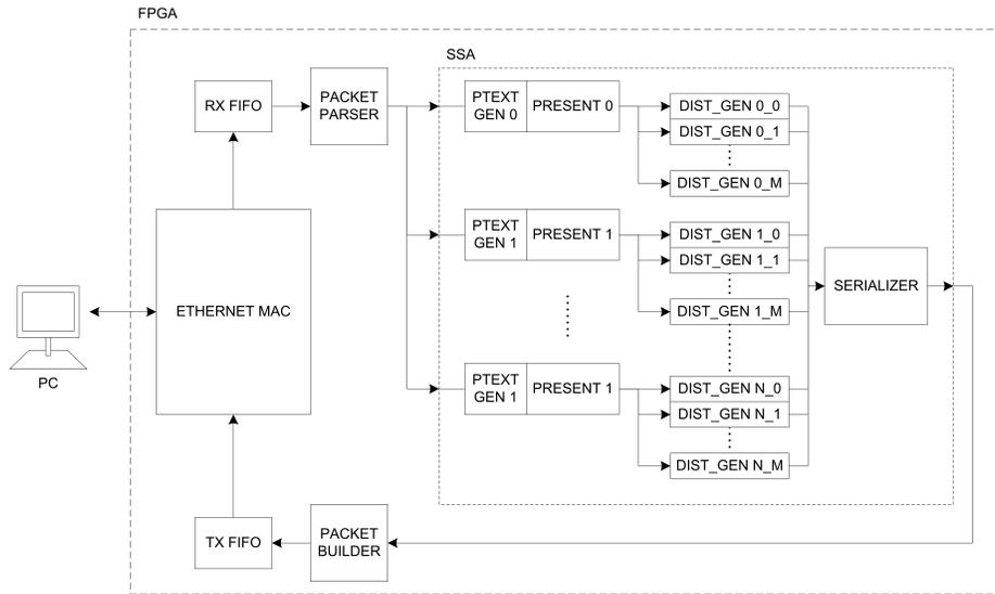
**Fig. 6.** Block diagram of the complete design
