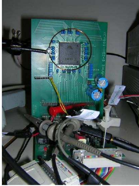
Figure 3.5: Measurement setup for EM attacks on FPGAs in the near field.
