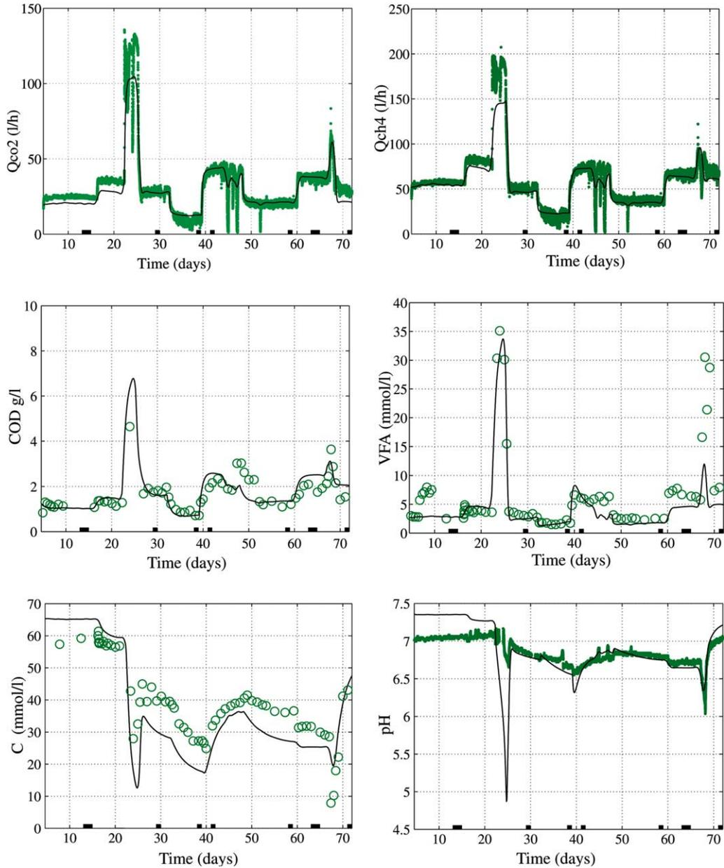
Fig. 7. Comparison between simulation results and measurements in a fixed bed anaerobic digester for the methane and CO<sub>2</sub> gaseous flow rates, pH, COD, VFA and total inorganic carbon (from [20]).
