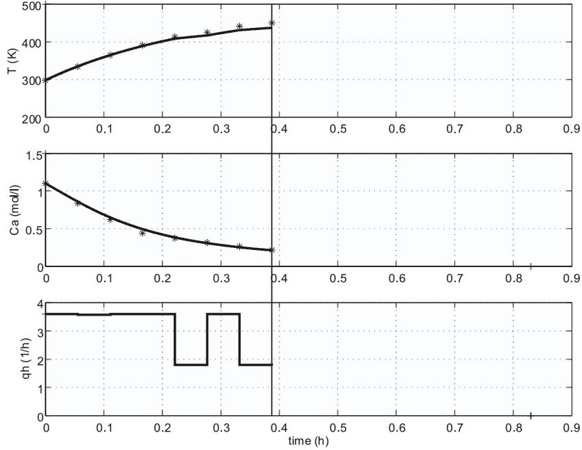
Figure 4.4: First piecewise linear approximation method. Evolution of the Temperature, the concentration and the heating rate for the heating task
