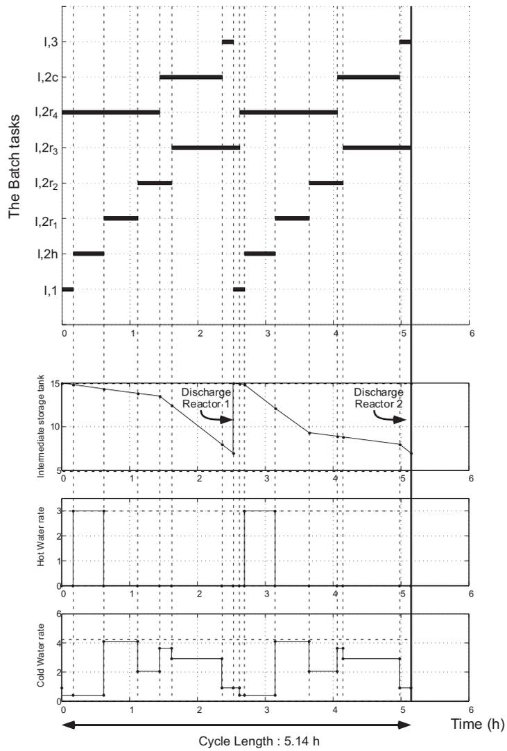
Figure 3.3: The scheduling of the batch tasks (2 reactors) and the evolution of the resources over the scheduling cycle
