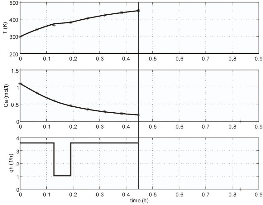
Figure 4.7: Trapezoidal method (14 time points). Evolution of the Temperature, the concentration and the heating rate for the heating task
