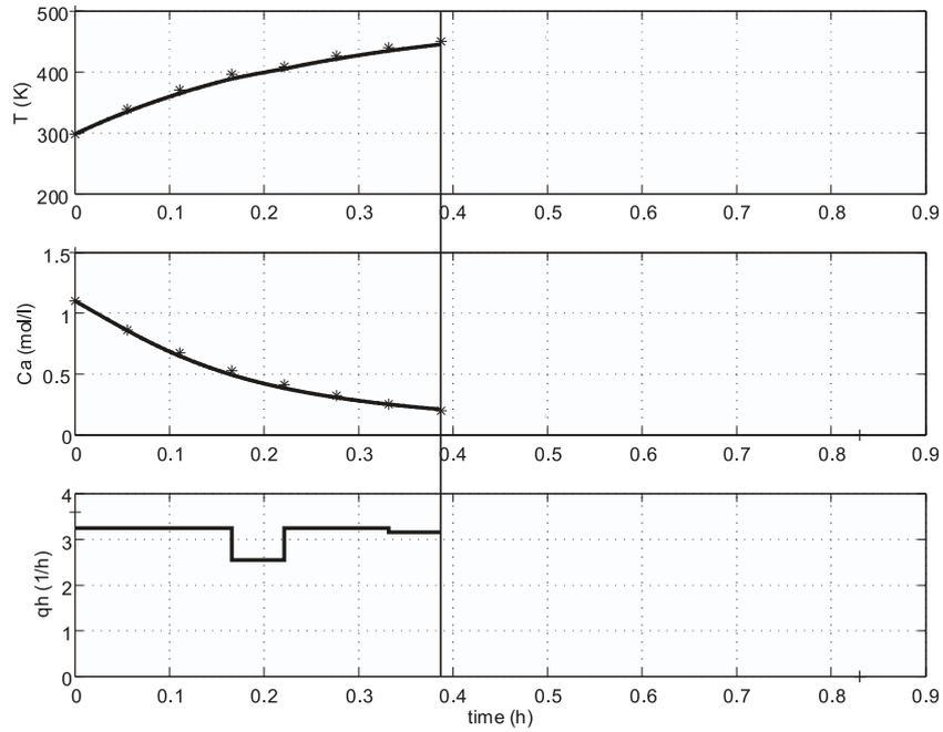
Figure 4.5: Second piecewise linear approximation method. Evolution of the Temperature, the concentration and the heating rate for the heating task
