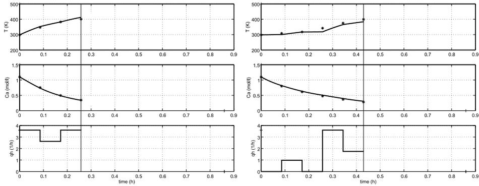
Figure 4.10: The trapezoidal method. Evolution of the Temperature, the concentration and the heating rate for the heating task on reactor 1 (left) and on reactor 2 (right).
