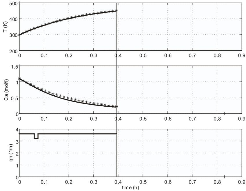
Figure 4.9: The second piecewise approximation method (56 time points). Evolution of the Temperature, the concentration and the heating rate for the heating task
