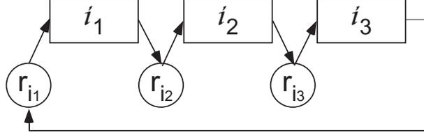
Figure 2.7: The resource task network for modeling the fixed sequence between batch tasks
