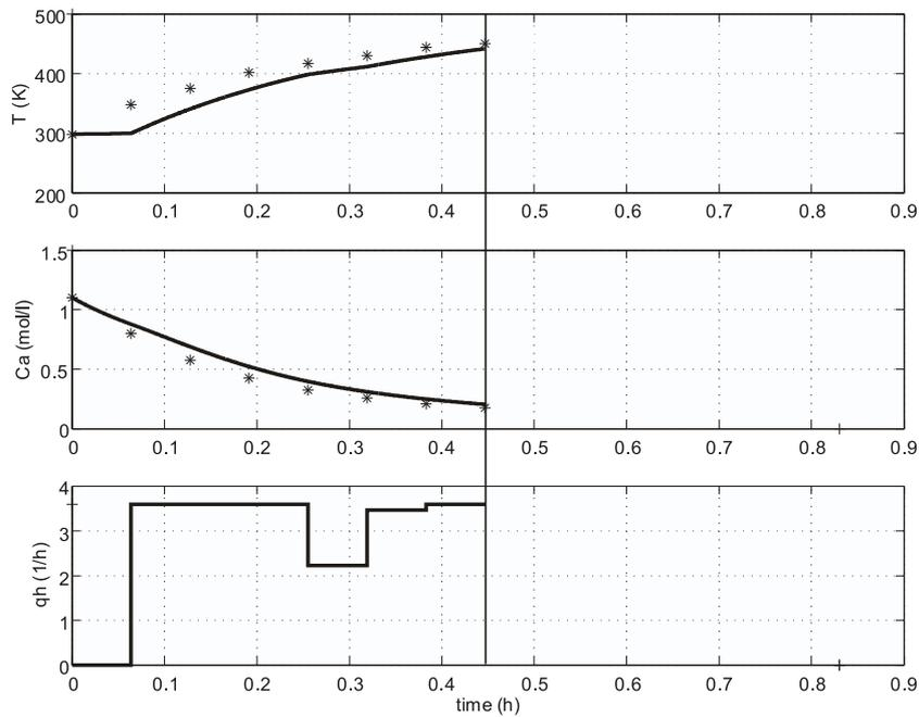
Figure 4.6: Collocation method (14 time points). Evolution of the Temperature, the concentration and the heating rate for the heating task
