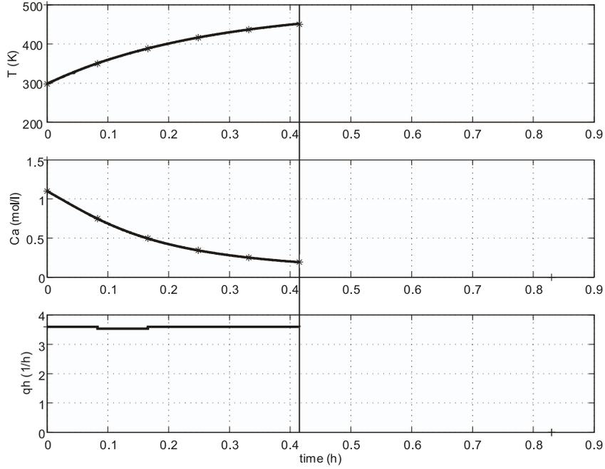
Figure 4.2: Collocation method. Evolution of the Temperature, the concentration and the heating rate for the heating task
