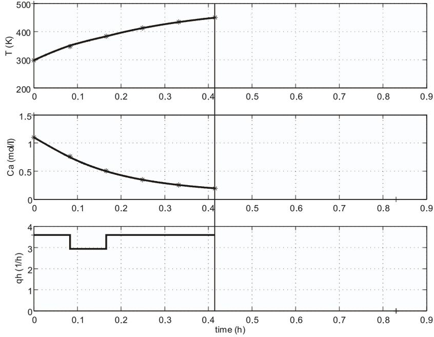
Figure 4.3: Trapezoidal method. Evolution of the Temperature, the concentration and the heating rate for the heating task
