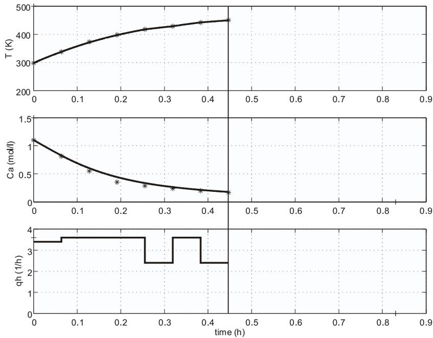
Figure 4.8: The first piecewise approximation method (27 hypercubes). Evolution of the Temperature, the concentration and the heating rate for the heating task
