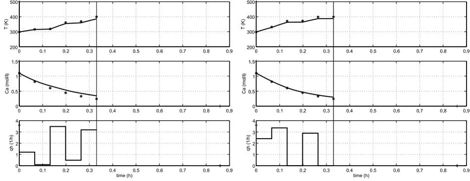
Figure 4.11: The second piecewise linear approximation method. Evolution of the Temperature, the concentration and the heating rate for the heating task on reactor 1 (left) and on reactor 2 (right).
