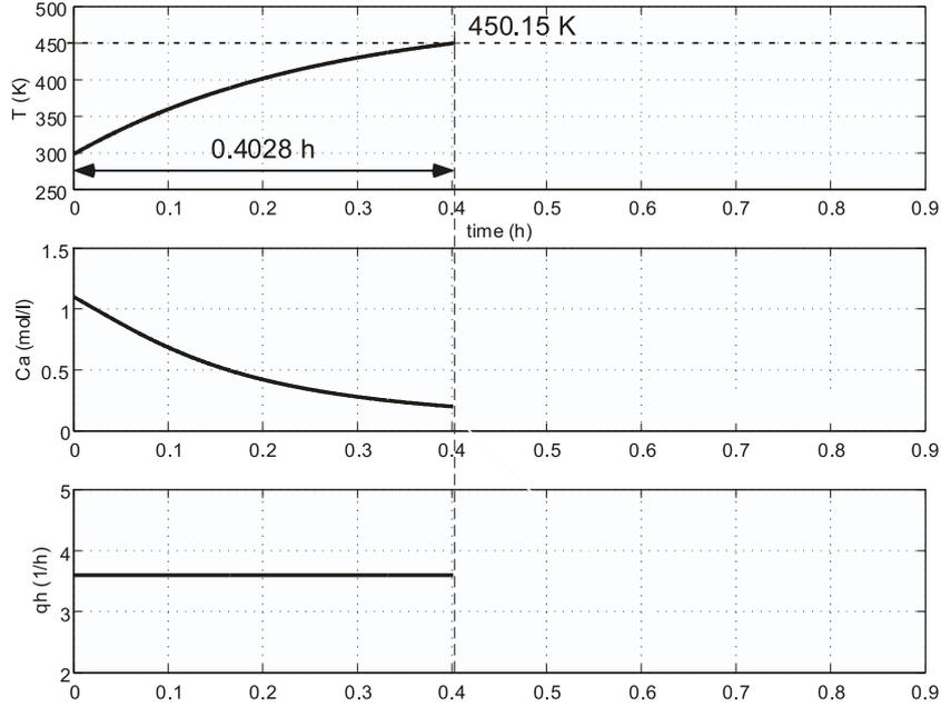
Figure 4.1: The optimal solution. Evolution of the Temperature, the concentration and the heating rate for the heating task
