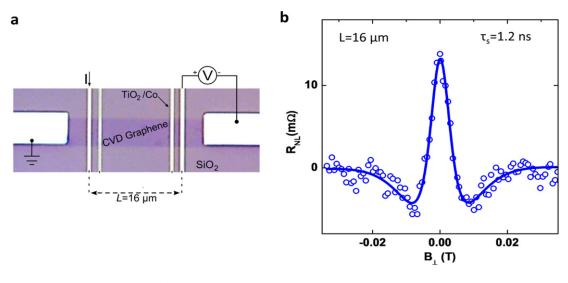
**Figure 4.** (a) Microscope image of a fabricated long-channel CVD graphene device on Si/SiO<sub>2</sub> substrate with multiple ferromagnetic tunnel contacts for spin injection and detection in a non-local geometry. (b) Hanle spin precession measurement in a L = 16  $\mu$ m long CVD graphene channel yielding spin relaxation time  $\tau_s$  of 1.2 ns at room temperature. Adapted from [16].
