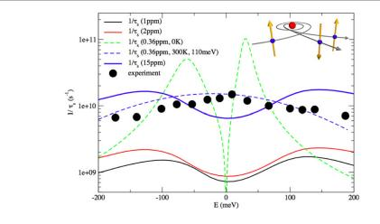
**Figure 7.** Energy-dependence of  $\tau_s$  derived from the *T*-matrix of the single impurity model at zero temperature (green dashed lines); and at 300 K broadened by puddles with energy fluctuations of 110 meV (blue dashed lines). Same quantity obtained from the real space spin propagation method for 1 ppm (solid black line), 2 ppm (solid red line) and 15 ppm (solid blue line) of H adatoms. Inset: schematic of the magnetic resonance process at the origin of enhanced spin relaxation.
