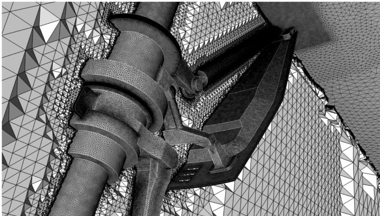
Figure : 3D with Boundary Layer mesh (10 million nodes).
