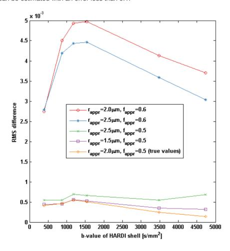
$\cdot$ 2) RMS signal difference vs b-value of a 90-gradient HARDI shells with  $\delta$ =15ms and  $\Delta$ =20ms. All the approximations use  $\alpha$ =67.5°, the value of the reference interwoven-fascicle signal..
