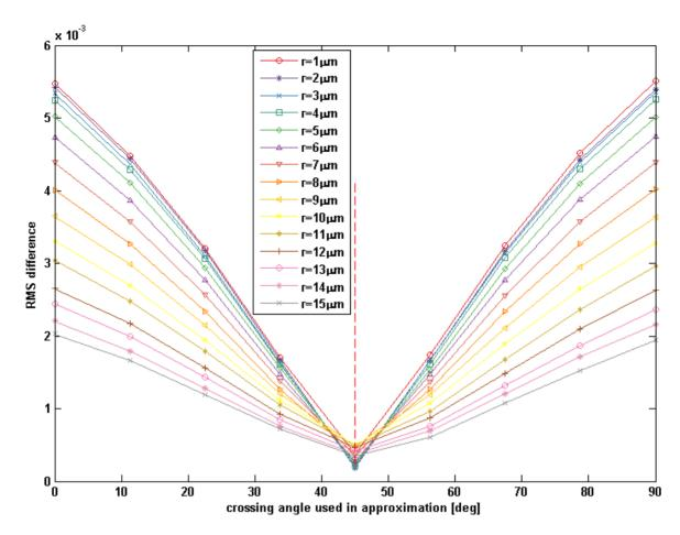
·3) RMS difference vs crossing angle, all other parameters kept equal. The reference angle is indicate by the red dashes. Reference density was 0.5.
