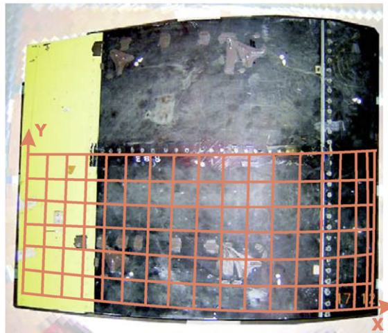
Fig. 3. Wing panel with superimposed impact grid.
