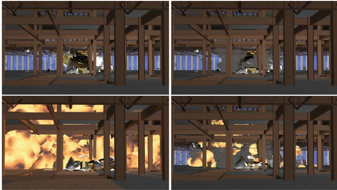
Fig. 2 Visualizations showing SPH model of the fuel and combustion in the building
