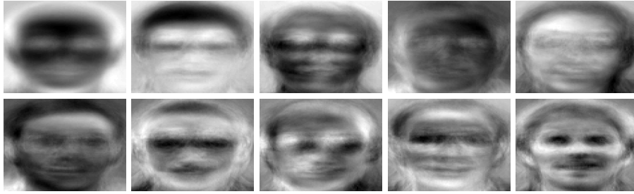
Figure 3: Left singular vectors (“eigenfaces”) for ORL Database of Faces computed via Algorithm 1 with rank k = 10 and updates of size l = 10 .
