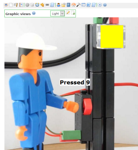
Fig. 4. HMI for a test setup with a switch and a lamp
