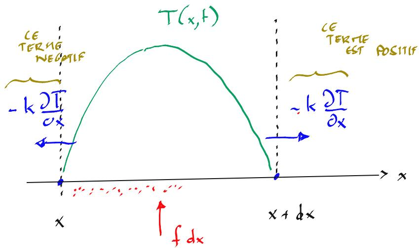
$$\rho c \frac{\partial T}{\partial t} = f dx + k \left. \frac{\partial T}{\partial x} \right|_{x+dx} - k \left. \frac{\partial T}{\partial x} \right|_x$$
