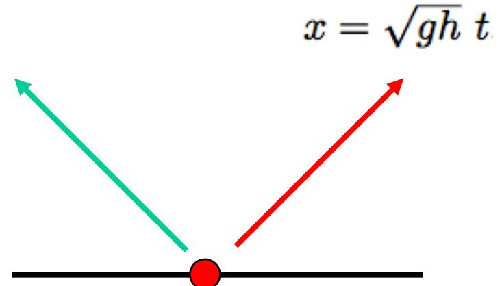
$$\begin{aligned} \left( \eta + \sqrt{\frac{h}{g}} u \right)^* &= r^* = r_L = \left( \eta_L + \sqrt{\frac{h}{g}} u_L \right) \\ \left( \eta - \sqrt{\frac{h}{g}} u \right)^* &= s^* = s_R = \left( \eta_R - \sqrt{\frac{h}{g}} u_R \right) \end{aligned}$$
