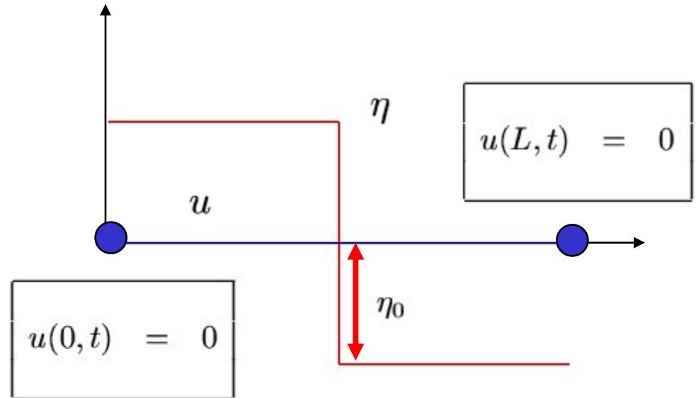
$$\begin{aligned}u(x, 0) &= 0 \\ v(x, 0) &= 0 \\ \eta(x, 0) &= \eta_0 & x \in [0, \frac{L}{2}[ \\ \eta(x, 0) &= -\eta_0 & x \in ]\frac{L}{2}, L]\end{aligned}$$
