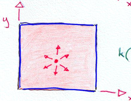
$$k \left( \frac{\partial^2 c}{\partial x^2} + \frac{\partial^2 c}{\partial y^2} \right) = 0$$
