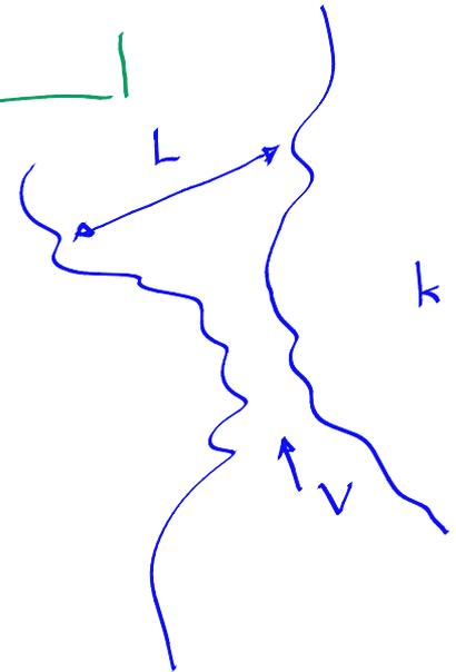
$$Pe = \frac{\text{red box}}{\text{green box}} = \frac{v \Delta c}{L} \frac{L^2}{k \Delta c} = \frac{vL}{k}$$
