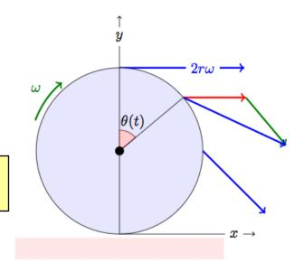
$$\vec{\mathbf{v}}(t) = \begin{bmatrix} v_c(t) \\ 0 \end{bmatrix} + r\omega(t) \begin{bmatrix} \cos(\theta(t)) \\ -\sin(\theta(t)) \end{bmatrix}$$
