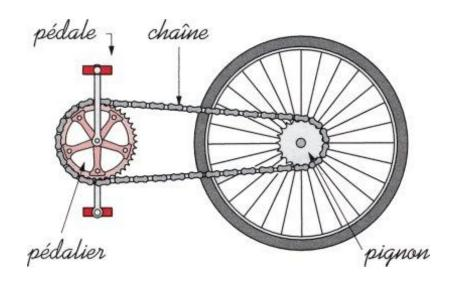
$$\underbrace{\omega_p r_p}_{v_p} = \underbrace{\omega_e r_e}_{v_e}$$
