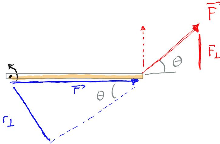
$$M_z = r_x F_y - r_y F_x = r F \sin \theta = F_{\perp} r = F r_{\perp}$$
