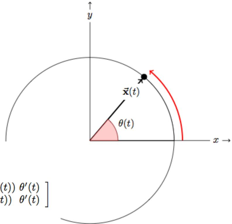
$$\vec{v}(t) = r \omega(t) \begin{bmatrix} -\sin(\theta(t)) \\ \cos(\theta(t)) \end{bmatrix}$$
