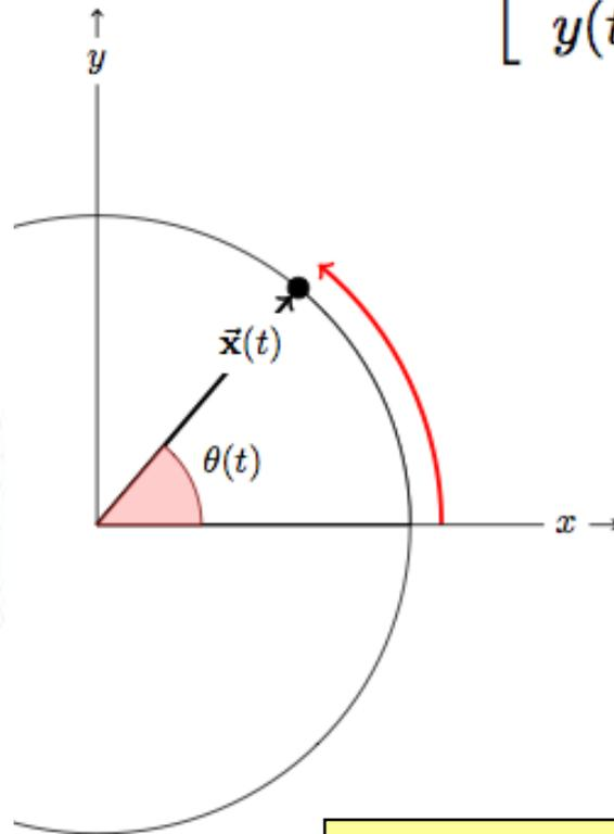
$$\begin{bmatrix} x(t) \\ y(t) \end{bmatrix} = \begin{bmatrix} r \cos(\theta(t)) \\ r \sin(\theta(t)) \end{bmatrix}$$
