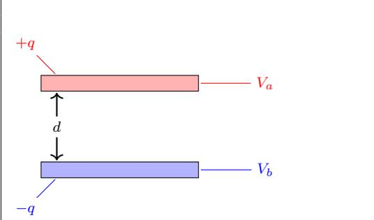
$$V_{ab} = V_a - V_b = \frac{d}{\epsilon_0 S} q = \frac{q}{C}$$
