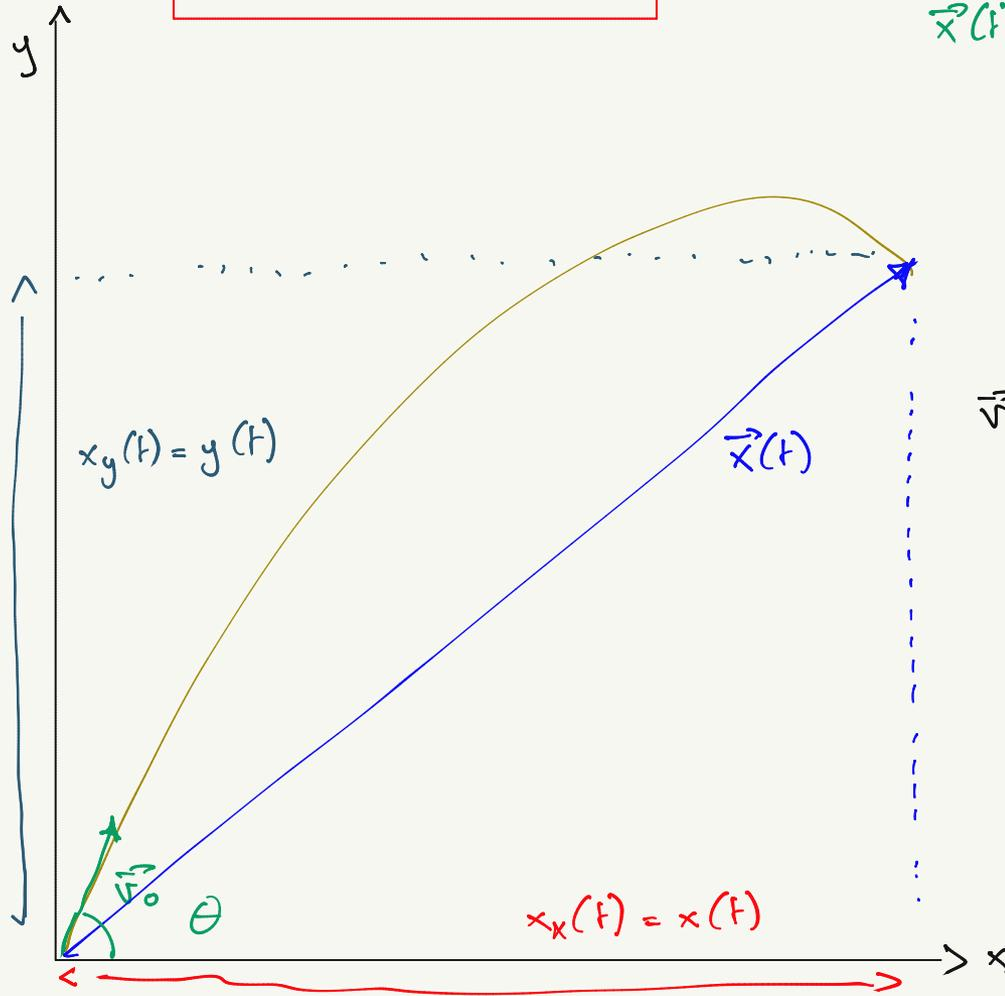
$$\vec{v}(t) = \frac{d\vec{x}}{dt} = \lim_{\Delta t \rightarrow 0} \frac{\vec{x}(t + \Delta t) - \vec{x}(t)}{\Delta t}$$
