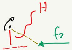
$$\left\{ \begin{array}{l} f_1 + f_2 = m \frac{v^2}{R} \\ N_1 + N_2 - mg = 0 \\ N_1 \frac{D}{2} - N_2 \frac{D}{2} + \underbrace{f_1 H + f_2 H}_{H(f_1 + f_2)} = 0 \end{array} \right.$$
