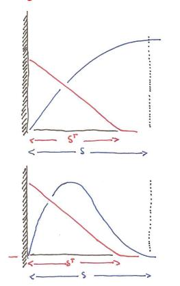
$$u \frac{\partial v}{\partial x} + v \frac{\partial v}{\partial y} = \beta g (T - T_0) + \nu \frac{\partial^2 v}{\partial x^2}$$
