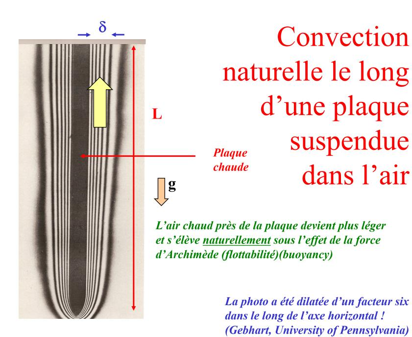
$$\rho_0(1 - \underbrace{\beta(T - T_0)}_{0}) \left( u \frac{\partial v}{\partial x} + v \frac{\partial v}{\partial y} \right) = \underbrace{\frac{\partial p}{\partial y}}_{\rho_0 g} + \mu \left( \frac{\partial^2 v}{\partial x^2} + \frac{\partial^2 v}{\partial y^2} \right) - \rho_0 (1 - \beta(T - T_0))g$$
