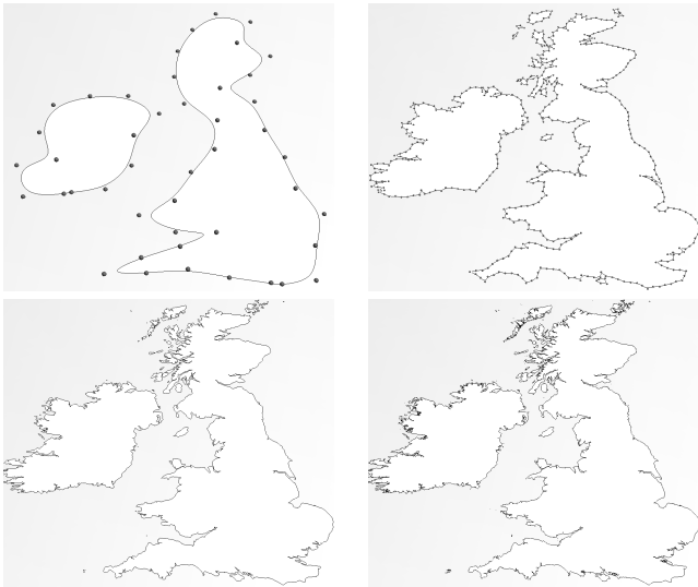
Fig. 5. Great Britain and Ireland with a resolution of 100 km (top/left), 15 km (top/right), 1.5 km (bottom/left) and 150 m (bottom/right). Splines control points are depicted on the geometry with the two lowest resolutions.
